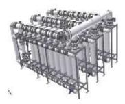
Ultrafiltration technology is used for the *separation of suspended solids, colloids, bacteria and viruses*. It is used as pretreatment for several processes such as reverse osmosis, ion exchange.
